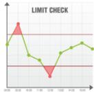
The standard limit check is performed when new data are acquired. This validation marks invalid values, which fall outside the specified range. This is a very simple but also very powerful tool sometimes referred to as technical validation. This type of validation is available as out of the box functionality, which can be used by user immediately after the solution is deployed.
